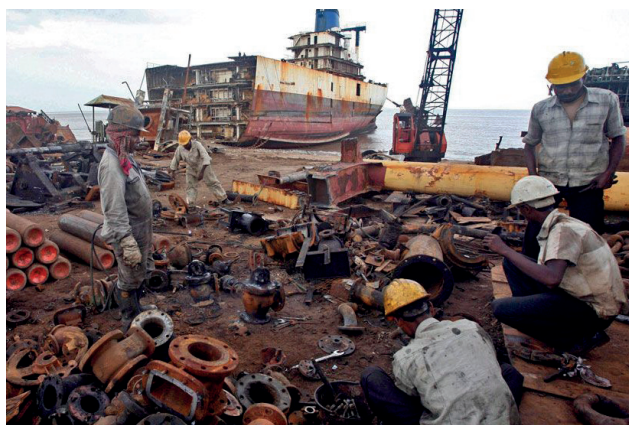
FIGURE 7. Beaching shipbreaking method
